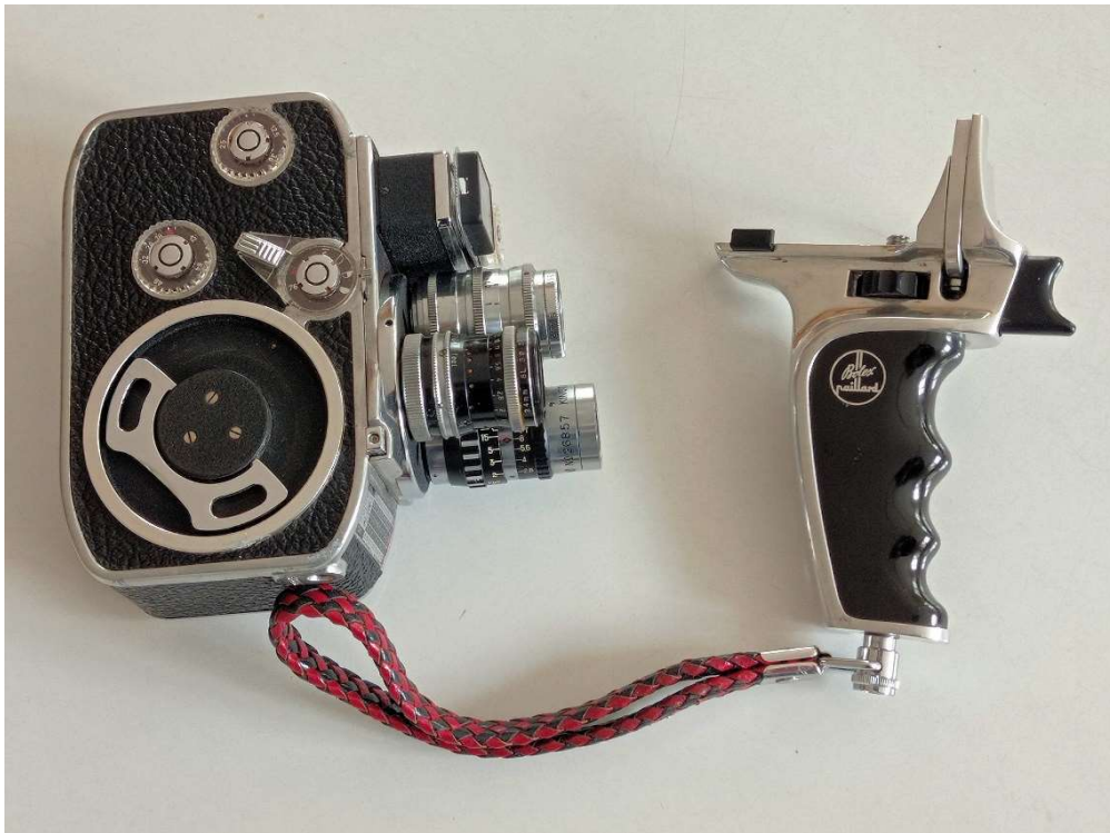
The Bolex D8 plus pistol grip. The wind-up handle for the spring is inside the large silver circle on the housing.
